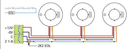
Multiple Detectors in Series Connection (using N/C Contacts) Individual wiring
